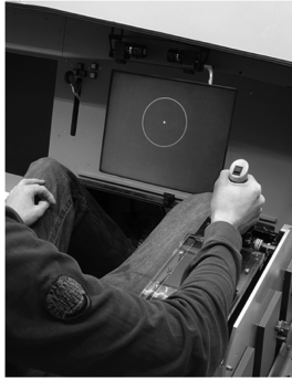
Fig. 12 Experimental setup showing display and side stick.
